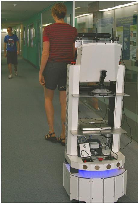
Figure 1: The experimental platform, a Mobile Robots Guiabot with Kinect sensor mounted on top of the touch screen
