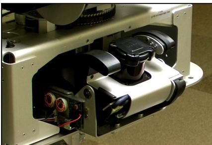
Fig. 3. Hokuyo laser mounted on a tilting platform.
