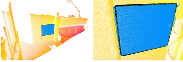
Fig. 7. The selected  $\mathcal{P}_s$  (represented with blue color) that potentially contains the door handle, based on a previously given door model, and the ADA door handle requirements.
